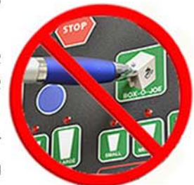
Do not use sharp objects to press the buttons on a switch.
